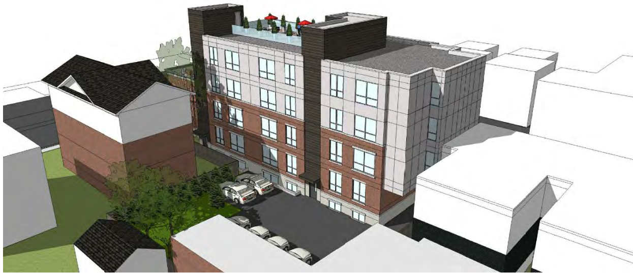
Figure 8: Model of the rear façade of the proposed development, illustrating the parking lot, green space, and rooftop outdoor space. (Roderick Lahey Architect Inc.)
