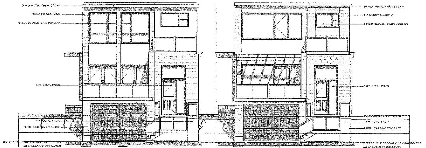
1 A-7 Front Elevation - Unit A 3/16" = 1'0"
