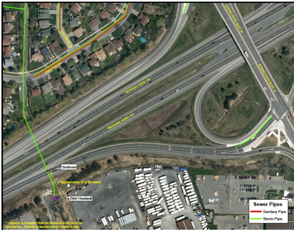
Figure 3 – 3.6 m Diameter Storm Sewer
